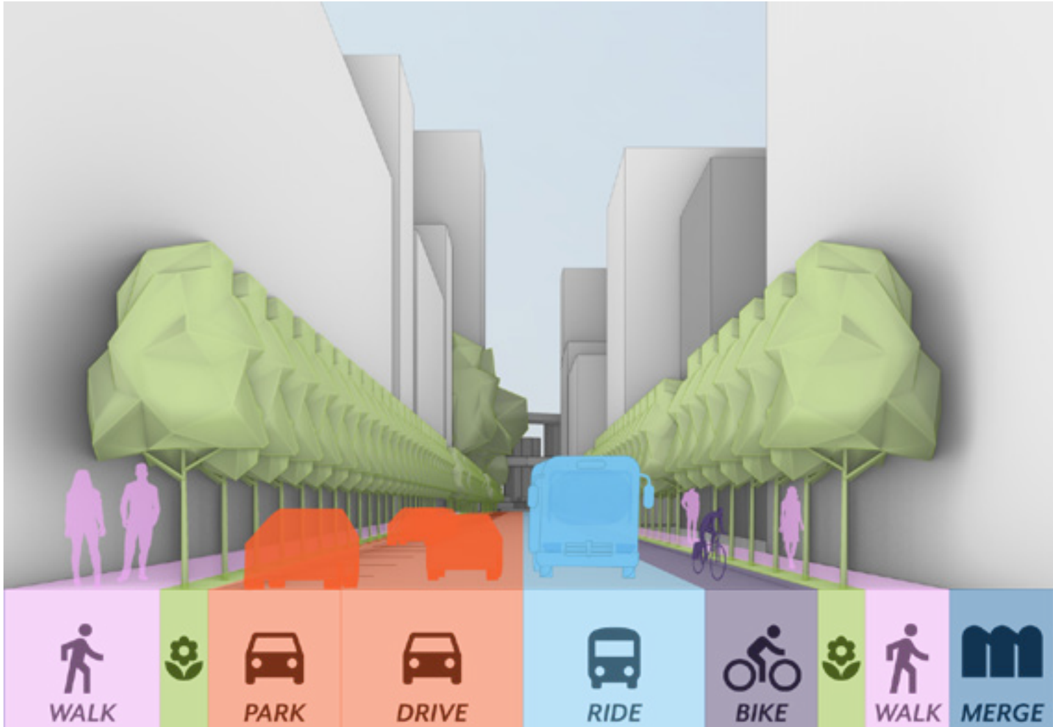
Proposed cross section of 7th Street with improved cycling infrastructure, street furniture, transit facilities and comfortable sidewalks.
